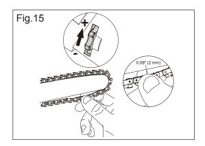
**NOTE:** New chains tend to stretch; check chain tension frequently and tension as required. **NOTE:** A chain tensioned while it is warm may be too tight upon cooling. Check the cold tension before next use.
