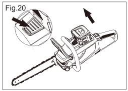
**NOTE:** Do not use force when installing the battery pack. If the battery pack does not slide in easily, it is not being inserted correctly.
