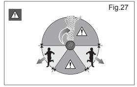
Make the felling back cut at least 5 cm. / 2 in. higher than the horizontal notching cut. Keep the felling back cut parallel to the horizontal notching cut. Make the felling back cut so enough wood is left to act as a hinge. The hinge wood keeps the tree from twisting and falling in the wrong direction. (See Fig.28)
