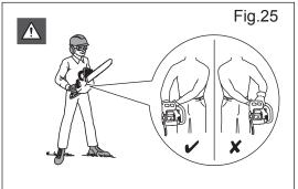
**WARNING:** Kickback may occur when the nose or tip of the guide bar touches an object, or when the wood closes in and pinches the saw chain in the cut. (See Fig.26)
