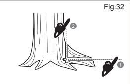
2. Remove the resulting loose section from the work area. Follow the correct tree felling procedure after you have removed the large buttress roots. (See Fig.33)
