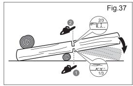
**NOTE:** When the log is supported on one end, cut 1/3 the diameter from the underside (underbuck). Then make the finished cut by overbucking to meet the first cut. (See Fig.38)
