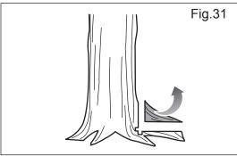
1. A buttress root is a large root extending from the trunk of the tree above the ground. Remove large buttress roots prior to felling. Make the horizontal cut into the buttress first, followed by the vertical cut. (See Fig.32)
