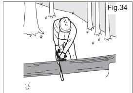
**WARNING:** Kickback may occur when the nose or tip of the guide bar touches an object, or when the wood closes in and pinches the saw chain in the cut. (See Fig.35)
