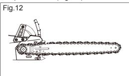
6. Slide the guide bar slot over the alignment flanges until the tension adjusting pin is inserted in the lower hole in the tail of the bar.
