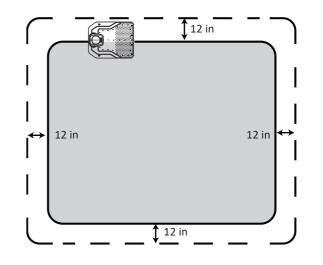
The recommended distance between two pegs is about 30 in in straight lines, and less in tight curves. Note that the pegs' hook and wire slit always faces the outside of the boundary. Within a short time the cable will be covered with grass. Since the voltage is only 32 V, there is no risk of electric shock. Make sure that the hook of the peg and the opening for the cable always face the demarcated.
