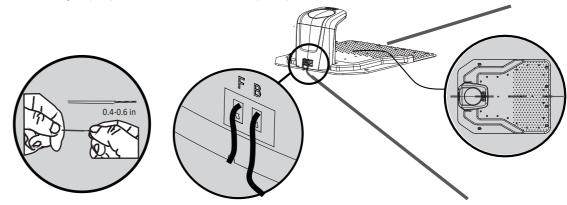
Insert the mains plug into a properly installed socket. Once the blue LED confirms all is OK, test the Robotic Mower's function. Check the LED regularly to ensure fixing the boundary wire has not affected the connection and signal shows S1 on the charging satation. Then place the Robotic Mower in the working area, a few metres beside the docking station. Set the main power switch to "ON". and then check the S1 signal on the panel is light on, press4 times 0 to unlock the panel.
