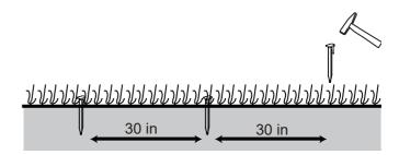
When first planting the pegs, do not drive them fully into the ground. Use a light hammer to drive them in a little bit. Also locate the fixing pegs and lay each one on the lawn at approximately the correct distance from lawn edges (12 in) and obstacles.
