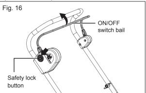
To stop the mower, release the On/Off switch bail.
