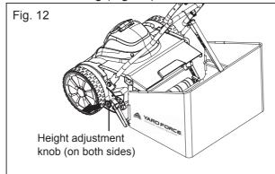
3. To adjust the reel to the highest cutting position, place the adjustment knobs through the top hole (position A) located on the sides of the reel mower frame. To adjust the reel to the lowest cutting position, place the adjustment knobs through the bottom hole (position B) located on the sides of the frame (Fig. 13).
