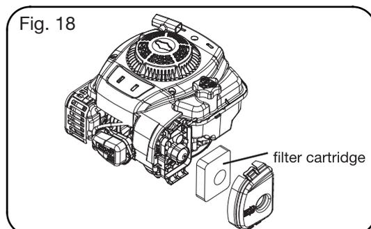
Soiled air filters reduce the engine output by restricting air to the carburetor. If the air contains a lot of dust, the air filter should be checked more frequently.
