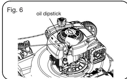
2. Remove the dipstick and check the oil level: the oil level must be between the Min and Max marks on the dipstick. If near the lower level, fill to upper level with the recommended oil (SAE30 or equivalent). Do not overfill. Wipe away any spilled oil align the ribs of the cap with the groove of the filler neck, then rotate to secure it (see Fig. 7).
